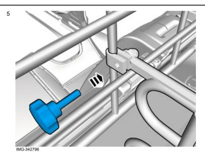
Only finger tighten the screw at this stage.
