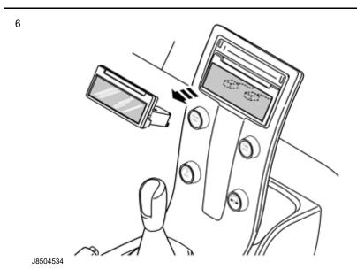
Press out the display from the rear of the centre console.
