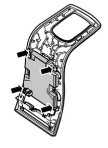
Remove the four screws for the dashboard environment panel.
