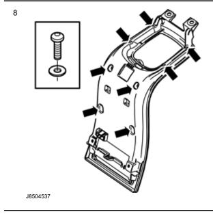
Remove the eight screws on the rear of the centre console. Remove the rear section.
