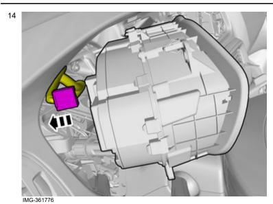
Disconnect the connector. The part is not to be reused.
