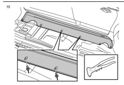
Rivet the panel through the two holes.
