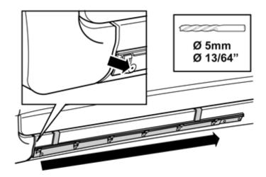
Drill out the six marked holes in the cradle using a Ø 5 mm (13/64") drill bit.
