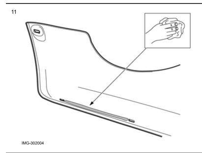
Clean the marked area on the protrusion between both mounting hooks on the front edge of the decor strip using isopropanol and wipe dry.
