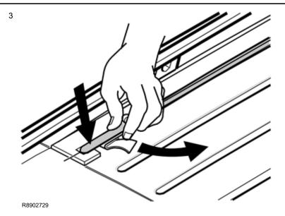
Take a roof protector rib from the kit (one at a time). Position the rib on the raised ridge along the edge of the guide moulding edge to edge with the rear end on the guide moulding cut-out
