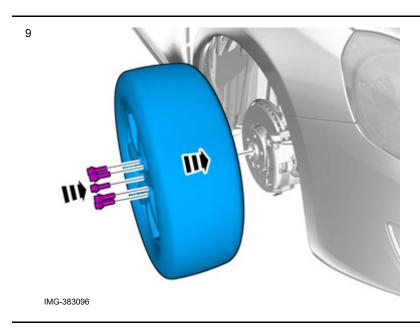
**Tightening torque:** Wheel to wheel hub Stage 1: 20 Nm Stage 2: 140 Nm
