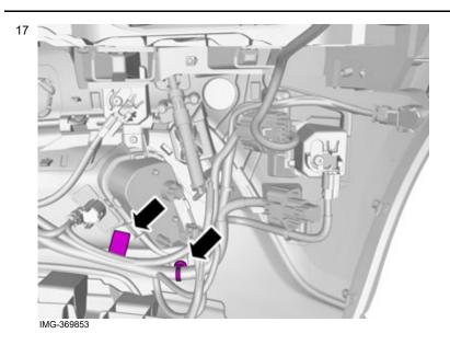
Remove the cable harness clips.
