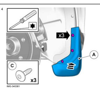
Clean the area where the mudflap is to be positioned.
