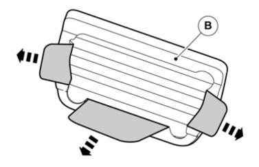
Hold the pedal protector as illustrated and fold out the three
