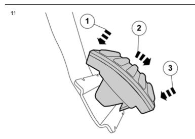
Hook the protector on at the upper edge, at the same time hold the tabs and pull downwards.
