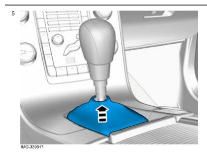
Move the boot and locking sleeve up so that the locking sleeve hooks into the gear shift knob.
