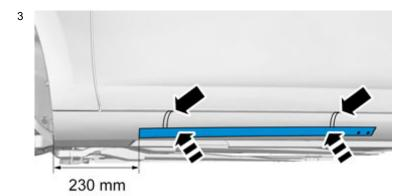
Align the front edge of the cradle according to the dimension measured from the front edge of the sill panel. Ensure that the tape does not adhere yet. Hook the cradle on the top of the sill panel.
