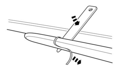
First pull off the protective tape at the panel ends towards the middle.
