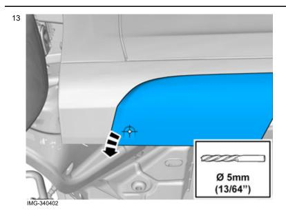
Fold the front edge of the plate around the lower edge on the sill panel properly and drill out the hole in the sill panel using a 5 mm (13/64") drill bit.
