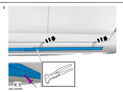
Rivet the cradle in all holes at the sill panel.
