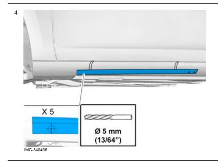
Drill out the five marked holes in the cradle using a Ø 5 mm (13/64") drill bit.
