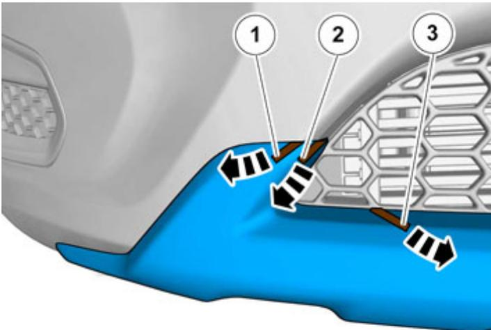
Carefully pull off the protective tape around both sides in the sequence shown, and secure each time.
