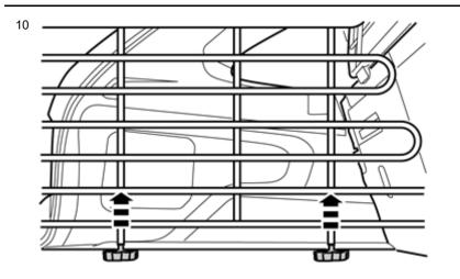
Adjust so that the cargo compartment wall is vertical and in the centre of the cargo compartment.
