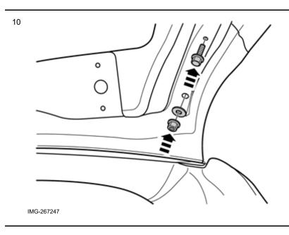
Take screws, washers and nuts from the kit. Tighten the spoiler to the boot lid.
