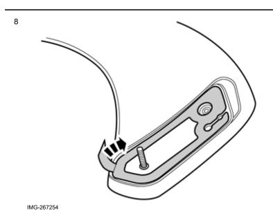
Remove the protective film from the tape on both feet of the spoiler.
