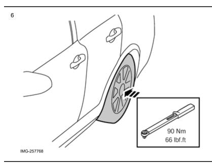
Reinstall the rear wheel, tightening torque 90 Nm (66 lbf.ft).
