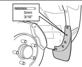
Drill a Ø5 mm (3/16") hole for the pop rivet.
