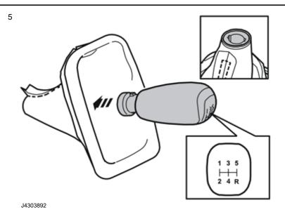
Guide the gear selector lever knob inside the out-turned gear selector lever gaiter. The text on the gear selector lever knob must point from the seam in the gaiter.
