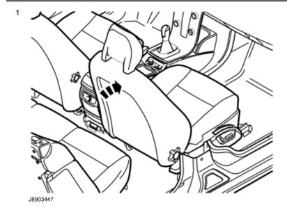
Fold the backrest forward on the front passenger side.
