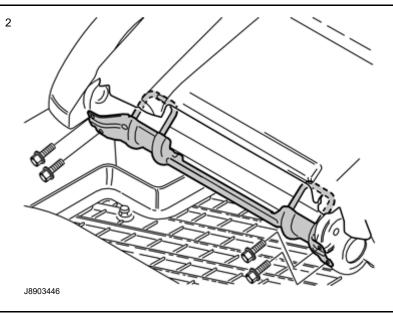
Install the ISOFIX attachment to the SIPS tube with the four screws from the kit. Tighten the screws to 10 Nm (7.5 lbf.ft.)
