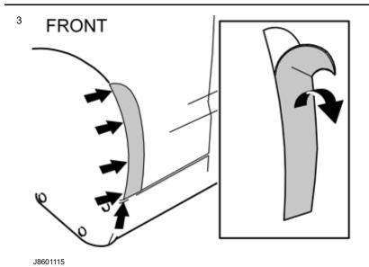
Remove the backing from the masking tape
