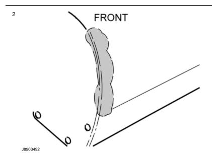
Clean the marked surface at the rear edge of the front wing. Use a mixture of 30% windscreen washer fluid and 70% water. Wipe dry.
