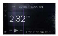
When weather data is not available, data such as temperature is replaced with - - "CURRENT LOCATION" will be the only visible information.
