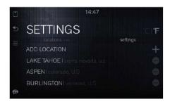
To remove a location, press the - (minus) icon on the right hand side of the location name. This icon rotates 90 degree and a delete button appear on the left hand side of the location name. To delete the location press the delete button and the item is removed from list. To cancel press the rotated minus icon on the right hand side. Current location is not available in settings because it cannot be removed.
