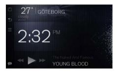
The SCT system goes into idle mode after 2 minutes if there is no interaction with the system. In idle mode a dimmed down version of the home screen is shown.
