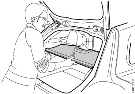
The locks are located on the cargo cover's underside.
