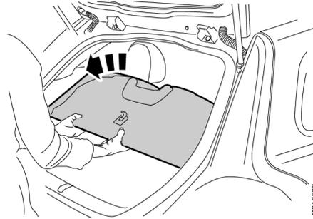
– Lift up the cargo cover at the rear edge and angle it down backwards.
