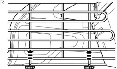
Tighten the knobs and secure the grille. The grille must be parallel with the floor hatch.
