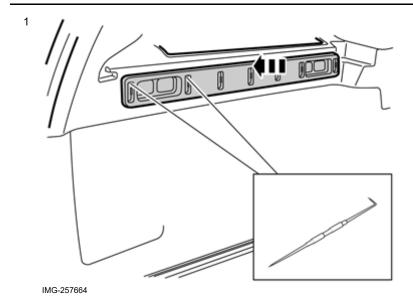
Take the left-hand rail (marked LH with the holes for attachment at the upper edge) and place the rear section in the hole for the rear load securing eyelet.
