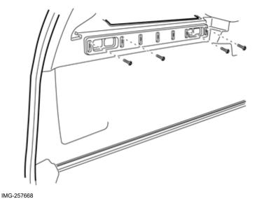
Align the rail, without the tape adhering, so that the four screws can be screwed into the side panel. The screws are self tapping and there may be some resistance when installing.
