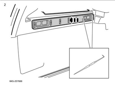
Align the front end of the rail carefully and make marks for the two front holes using a scriber.
