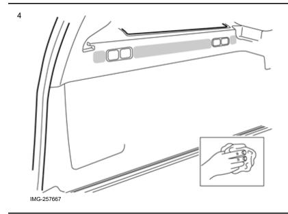
Clean the marked surfaces using a mild, not etching, cleaning agent and wipe dry.
