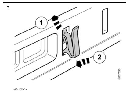
Install the hooks by inserting them in the upper edge (1) and then downwards (2) until they lock in the rail.
