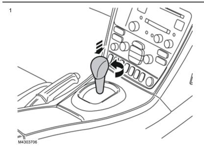
Press the gear selector lever knob down and twist a  $\frac{1}{4}$ turn to the left
