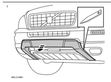
Detach the existing bumper by carefully prizing at the lower edge, between bumper and bumper cover, using a plastic weatherstrip tool. Following which, pull the bumper straight out so that the catches release.
