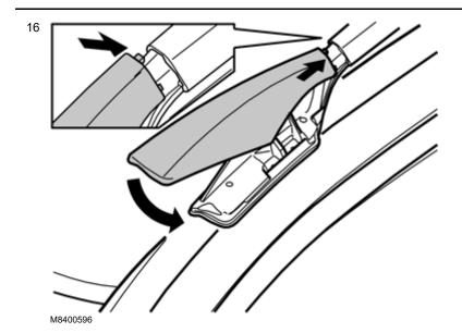
Install the cover on the front mounting for the rail
