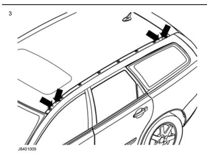
Remove the four screws in the roof joint and put them to one side. They will not be used again
