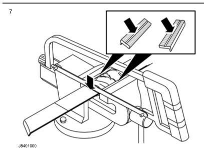
Wrap the section of the roof trim to be secured in the vice. Use plenty of paper or cloth to protect the paintwork on the roof trim
