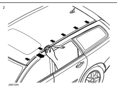
Remove the roof trim (it is secured by eight clips). First grasp the inside using the finger tips of one hand and pull it out towards the edge of the roof. Then, use the other hand to carefully pry up the outer side using a plastic weatherstrip tool. Unhook the roof edge trim from the clips.
