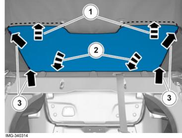
Press the shield in to place between the roof panel and window and in the clips.
