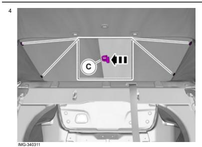
Position the clips between the rear window and panels approximately in the positions shown.
