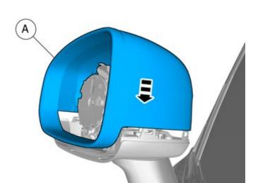
Install component that comes with the accessory kit. Ensure that all clips engage.
