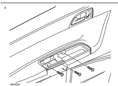
Remove the three screws holding the door panel to the side of the door.
