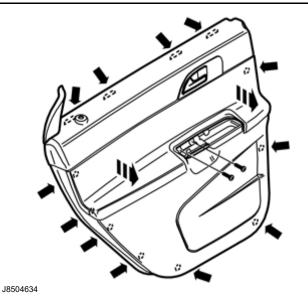
Remove the two screws holding the door panel to the side of the door.
