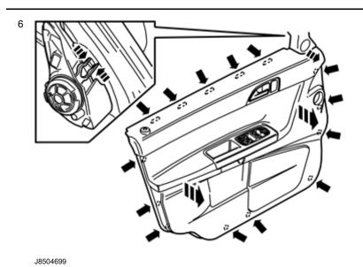
Detach the door panel from the side of the door by carefully prizing it away opposite the nine clips at the sides and furthest down using a weatherstrip tool.
