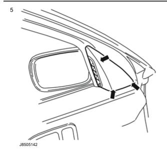
Remove the small panel at the front edge/top edge of the door. Carefully prize it away using a weatherstrip tool, opposite the three clips.
