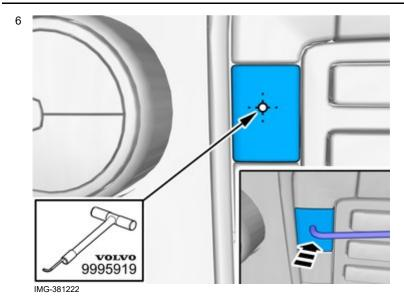
**Use special tool:** T9995919, PULLER (SEAL-PINION,CAM-CRANKSHAFT)B200-6304
