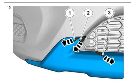
Carefully pull off the protective tape around both sides in the sequence shown, and secure each time.
