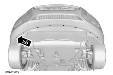
Remove the screws and place to one side. New ones can be found in the kit.
