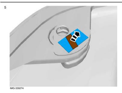
Remove the backing tape from both templates.
