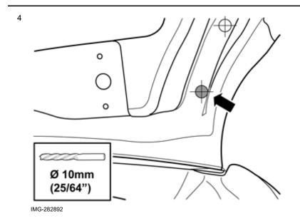
Drill out the upper/front hole. Use a Ø 10mm (25/64 ")drill bit.
