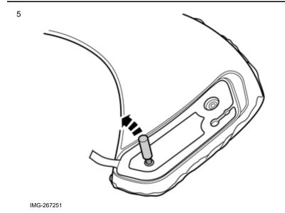
Remove the protective covers from the spoiler's studs on both sides.
