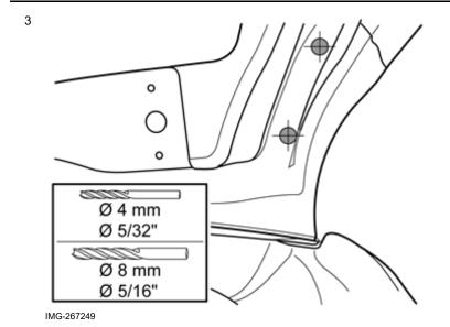
Pre-drill the holes using a Ø 4mm (5/32 ") drill bit (part.no. 9814090) in the punched holes. Then drill out the holes using an Ø 8 mm (5/16 ") drill bit. Drill at right angles to the surface.
