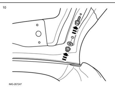
Take screws, washers and nuts from the kit. Tighten the spoiler to the boot lid.
