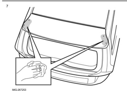
Clean the boot lid at the markings where the spoiler's feet are to be positioned. Use isopropanol and then wipe dry. Compare the surface with the spoiler's feet so that the surface is sufficiently cleaned.
