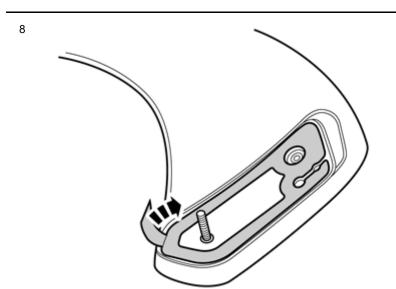
Remove the protective film from the tape on both feet of the spoiler.
