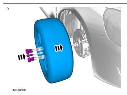
**Tightening torque:** Wheel to wheel hub Stage 1: 20 Nm Stage 2: 140 Nm
