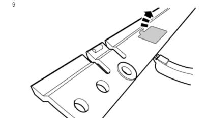
Remove the protective tape from the mounting tape on the front holder.
