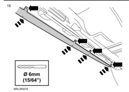
Press in the sill decor opposite the mounting eyelets against the underneath of the door sill panel. Drill out the holes through these using a  $\emptyset$ 6 mm (15/64") drill bit. Remove any swarf.
