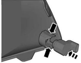
Install the sensor in the new panel. Ensure that the catches engage.
