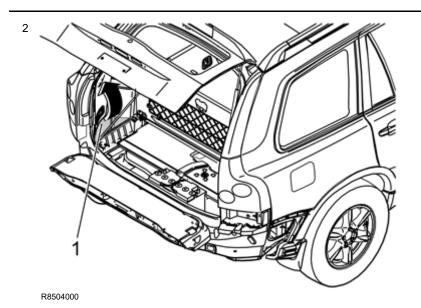
Remove the left-hand side floor hatch (1).
