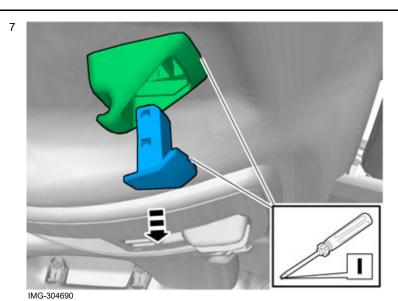
Applies to mirrors without autodim Carry out on both sides.
