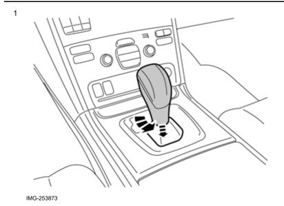
Loosen the gaiter from the gear lever knob by turning the lock ring on the inside  $\frac{1}{4}$ -turn, and pull down the gaiter.
