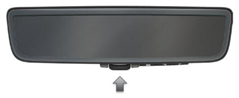
Push lever forward and adjust mirror so that vision out the rear window is normal.
