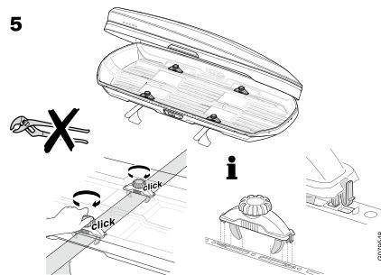
Make sure that the clamps are installed properly as illustrated
