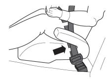
If the shoulder belt touches the neck, then place both the lap and the shoulder belt under the corner. Then go back to point (7). If the shoulder belt is below the shoulder even though it is located across the corner, the child has outgrown the child restraint. 13.
