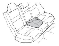
Place the booster cushion on a seat with approved continuous-loop lap and shoulder belt.
