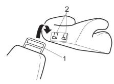
Place the backrest adjustment bar (1) in the cushion's tension mounting yoke (2).
