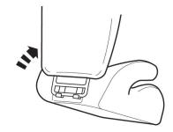
Turn the backrest so that the upper crossmember of the adjustment bar engages into the upper part of the tension mounting yoke.
