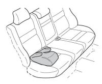
Place the booster cushion on a seat with approved continuous-loop lap and shoulder belt.
