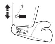
Raise or lower the backrest by pressing the button (1) on the back of the backrest. There are five fixed positions.
