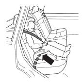
Position the child and tighten the lap belt's fixed end under the corner of the booster cushion. 7.
